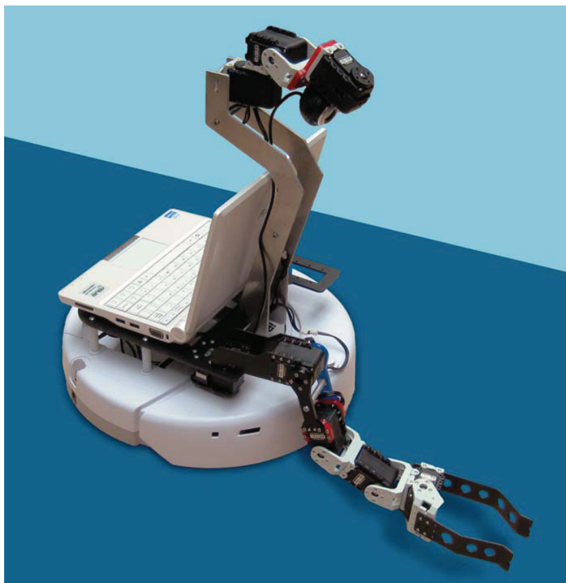
Calliope: A prototype Create/ASUS robot with a pan/tilt camera and gripper arm.
