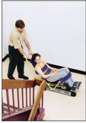
4. Turning at the Landing It is recommended to use the inside of the stairway to allow room for other traffic and to make it easier to turn corners at stairway landings. To turn the Evacu-Trac on flat surfaces, the attendant pushes down on the handle and pivots the unit on the rear auxiliary wheels.
