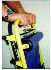
6. Evacu-Trac Fail Safe Brake The Evacu-Trac brake is normally on. To descend the stairs, release the brake by slowly squeezing the brake lever. Descent speed can be slowed by reducing pressure on this lever. A governor limits the maximum descent speed to about 3' per second, allowing even a small attendant to safely transport heavier riders.
