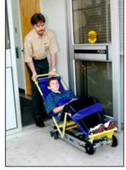
5. Moving on Flat Surfaces Once clear of the emergency area, park the Evacu-Trac on a flat surface and engage the brake by releasing the bar.
